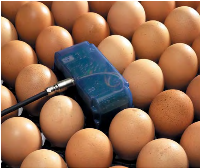
Fig.1 - OvoScan™ monitors the actual eggshell temperature on-line and continuously adjusts the incubator temperature in order to achieve the required eggshell temperature trajectory.
